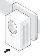
More: To add additional Powerline adapters and extenders with the default settings, simply plug them into the wall sockets on the same electrical circuit.
